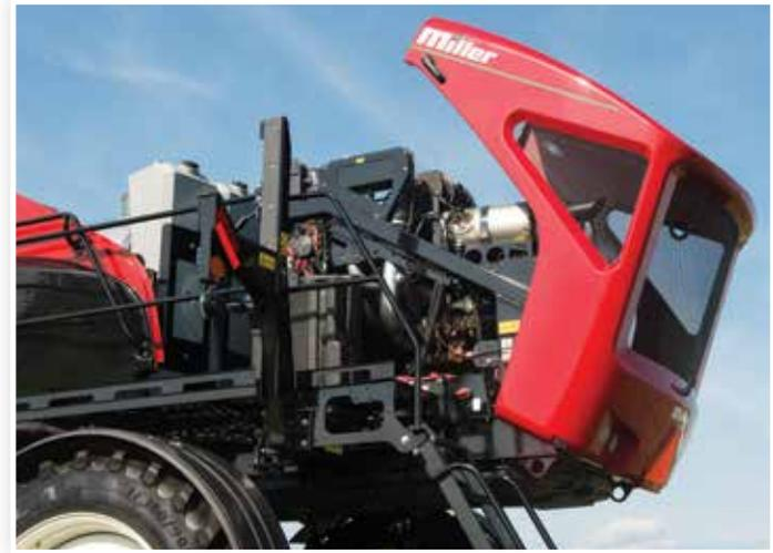
Engine and hydraulic service checkpoints are easy to access from the walkway by the engine compartment.
